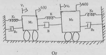
(b) Obtain the transfer function using Mason's Gain formula for the system given.
